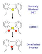
The MRTI research team has reproduced this sulfur removal reaction in the laboratory below 200 degrees C at atmospheric pressure. The first potential application of this technology is likely diesel desulfurization. Beyond this first application, this technology could be developed further for application at the wellhead for heavy feeds, significantly reducing cost and increasing the efficiency of sulfur removal.
